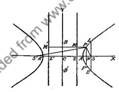
Since e > 1, the line SZ can be divided internally and externally in the ratio e : 1. The points of division A and A' clearly lie on the hyperbola.
