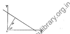
The intercepts which this line makes with the co-ordinate axes are obviously  $p \sec \alpha$  and  $p \csc \alpha$ . Proceeding as in case 3, the equation to the line will be seen to be
