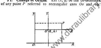
Let O' be the point (h, k) and O'X and O'Y lines drawn parallel to Ox and Oy respectively. Let (X, Y) be the co-ordinates of P referred to O'X and O'Y as co-ordinate axes. If then straight lines are drawn parallel to these axes, it is easily seen that
