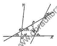
If P be any point (x, y) on the line inclined at an angle  $\theta_1$  to the axis of x and cutting off an intercept  $c_1$ from the y-axis, the triangle PRQ, where PR and QR are drawn parallel to OY and OX, gives
