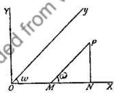
Let the co-ordinates of a point P be (x, y) referred to oblique axes OX, Oy, and (X, Y) referred to rectangular axes OX, OY.
