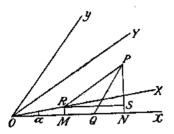
Mary.org.in Let  $\omega$ ,  $\omega'$  be the angles between Ox, Oy and OX, OYrespectively and  $\alpha$  the inclination of the new x-axis to the old. Let the co-ordinates of any point P be (x, y) and (X, Y) referred to old and new axes respectively.
